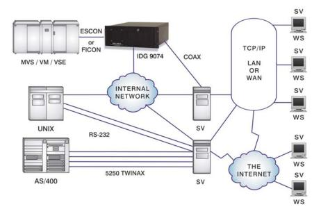
SV = SuperVision Server SV WS = SuperVision Workstation IDG 9074 = IDG 9074<sup>®</sup> Secure Communications Controller<sup>®</sup>
